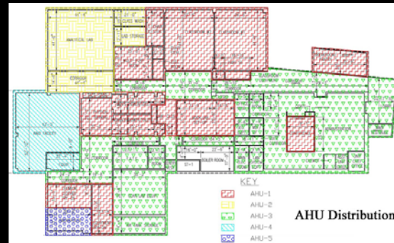
FIVE AHU'S IN MECHANICAL MEZZANINE
